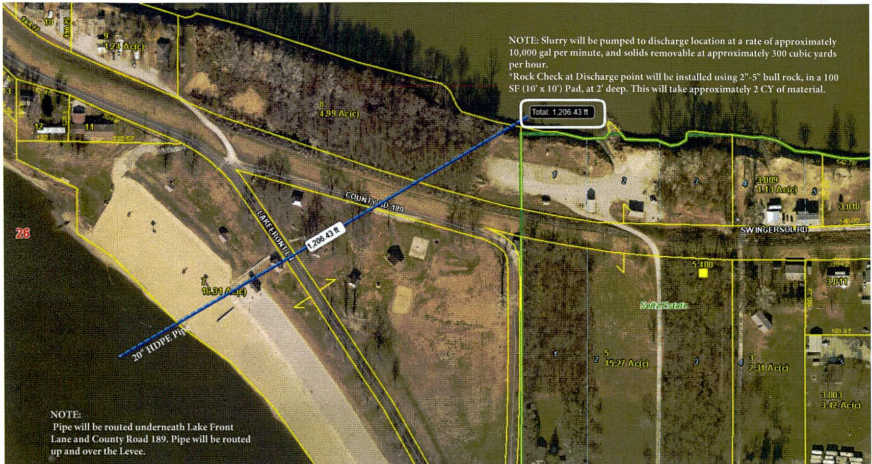
FIGURE 2 OUTFALL LOCATION AND DREDGING INFORMATION
